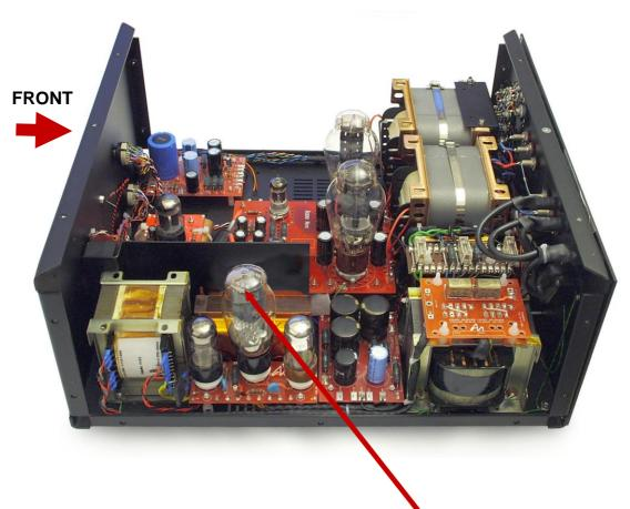
Looking from the front of the amplifier, insert the **5U4G** valve into the last empty socket located on the right, situated between two smaller valves. Locate the rib on the central pin of the valve and align with the valve base (it can only be inserted one way due to this locating rib) and with gentle but firm pressure insert the valve.
